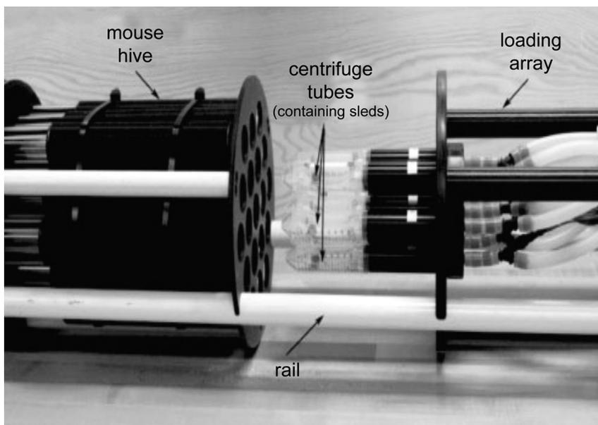
**Fig 6.** Multiple mouse MRI loading system described by Dazai et al.<sup>22</sup> Mice loading array equipped with anesthesia and a mouse hive, which holds up to 19 receiver coils. Reproduced from Dazai et al<sup>22</sup> with permission from John Wiley and Sons.
