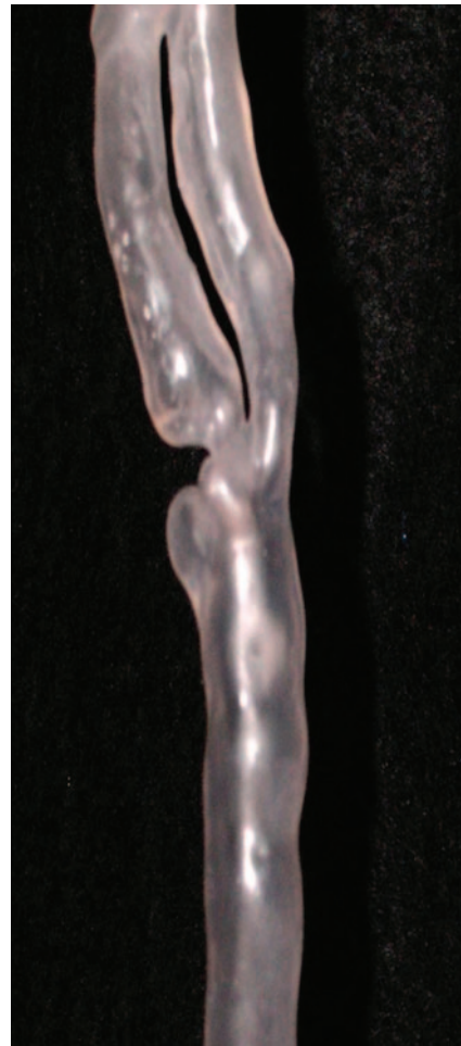
FIG 3. Silicon replica made by the lost-wax technique. This replica was then used to study the flow dynamics of this patient by placing it in a neck phantom and perfusing non-Newtonian fluids while injecting isobaric dyes into the slipstreams (not shown here). The replica was next placed into the scanner, the fluid in the phantom was made isoattenuated to the silicon with contrast agent, and the entire phantom was scanned by using the same scan parameters as were used to scan the patient.
