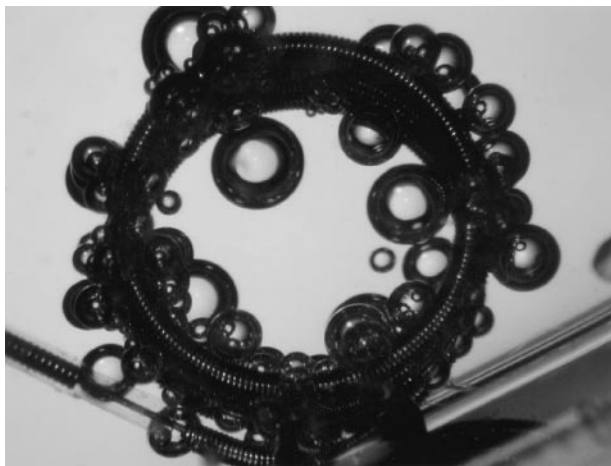
FIG 1. Depiction of the detachment process of a conventional coil (GDC-10, 4 mm \times 10 cm) in saline. Many gas bubbles were generated from the coil and attached around the entire coil part. The bubbles varied in size.
