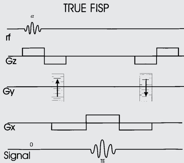
FIG 12. True FISP sequence structure with balanced gradients. Net effect of gradients allows spins that are stationary as well as those moving with constant velocity to reach a steady state.  $G_z$  = slice select gradient,  $G_y$  = phase encode gradient, and  $G_x$  = frequency encode gradient.
