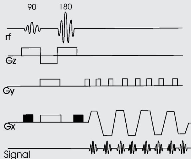
FIG 1. EPI diffusion-sequence structure. The 90° and 180° RF pulses are followed by a bipolar, trapezoidal frequency encode gradient (Gx) for rapid collection of multiple echos. DWI is applied by symmetrical gradients along a frequency-encoded direction (black rectangles). Subsequent sequence acquisitions would apply diffusion weighting along phase (Gy) and slice-select (Gz) directions.
