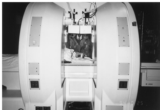
FIG 3. Patient in supine position within vertical gap of the open-configuration magnet with mounted display monitors (arrows) above.
